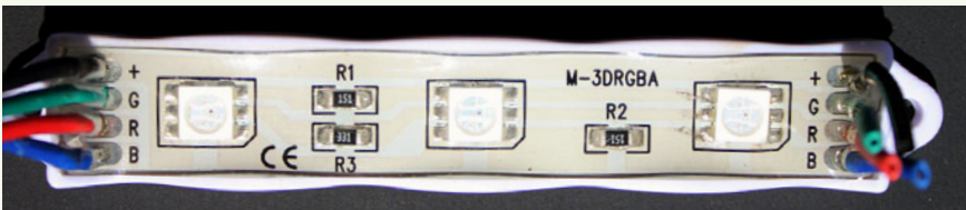
5050 LED's with Varying RGB Color Rendering and Effects
